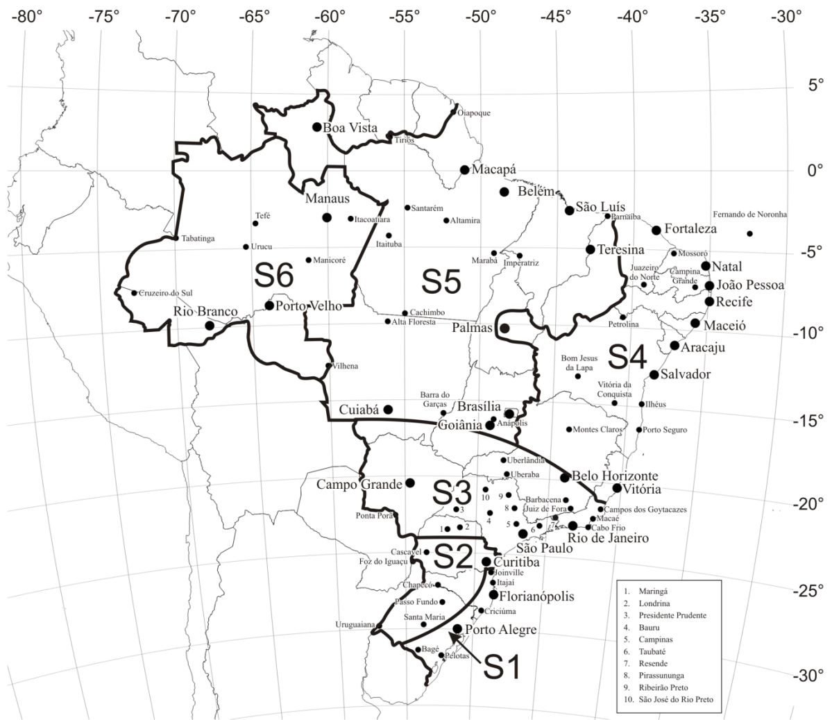
Figure I.5 – Definition of zones for Type S extreme winds (synoptic).
