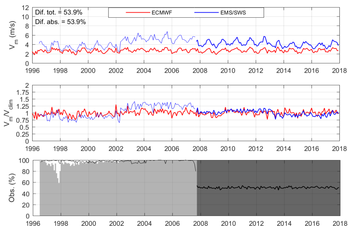
Figure 6.12 – Monthly mean wind speeds for SWS and ECMWF data for SBCG – Campo Grande, MS (top); monthly means normalised by V_{clim} (middle); percentage of month with valid observations (columns), with percentage of even numbered observations in knots (line) (bottom).
